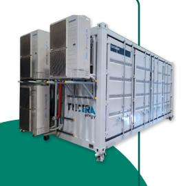
The **TRICERA 24ft HC storage unit** is a compact 1500 V design, efficiently housing batteries, a battery control and energy management system, HVAC system, and extensive safety features, suited for all environmental conditions. The batteries can be configured for up to **4.15 MWh** for use in various applications. Several different battery to-
